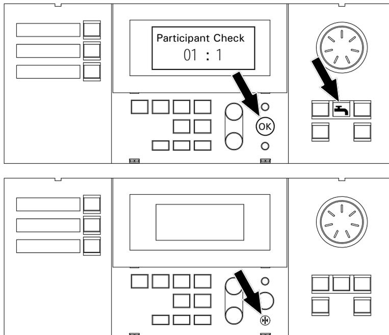
participant flash and the words “Check OK” should appear in the screen of the Cascade control. If the communication confirms to be OK, then the connection is correct. Devices such as the Output Module will have a green LED which will flash for confirmation of the check.
